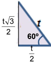
$$\text{sen } 60^\circ = \frac{\text{cateto oposto}}{\text{hipotenusa}} \rightarrow \text{sen } 60^\circ = \frac{t\sqrt{3}}{2} \div t \therefore \text{sen } 60^\circ = \frac{\sqrt{3}}{2}$$
