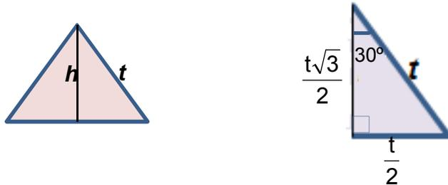
$$\text{sen } 30^\circ = \frac{\text{cateto oposto}}{\text{hipotenusa}} \rightarrow \text{sen } 30^\circ = \frac{t}{2} \div t \therefore \text{sen } 30^\circ = \frac{1}{2}$$
